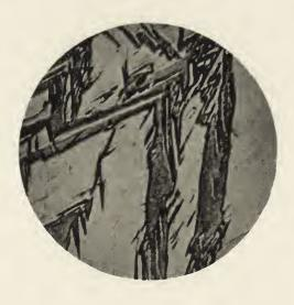
Fig. 12. Steel containing 1.5 per cent. C., quenched in ice water.
